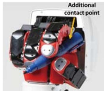
写真2 Stabilized cylindrical tool handling using additional contact point
